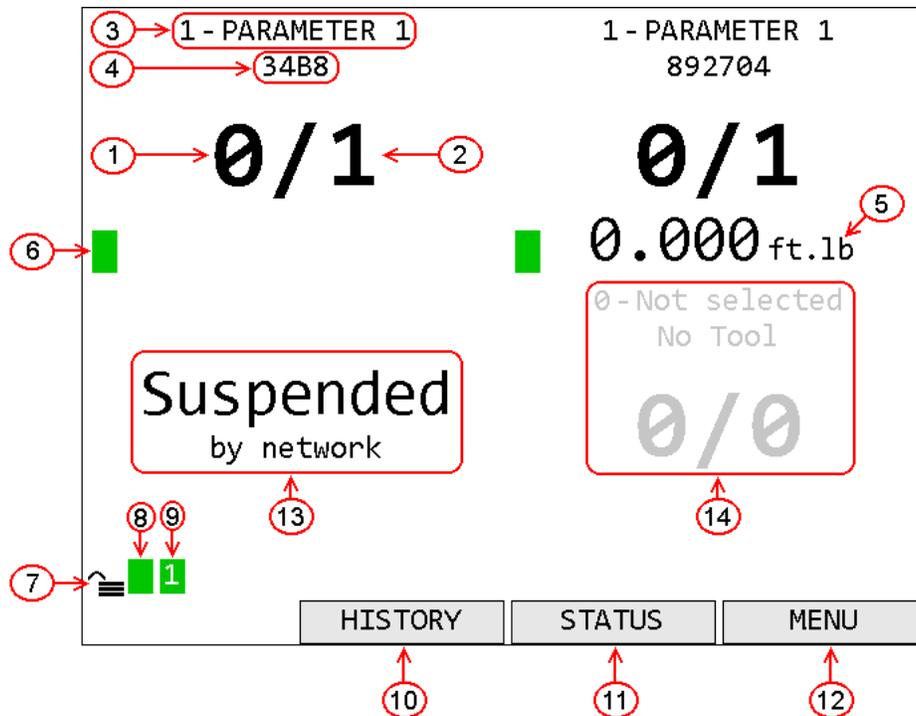
1. Count – The number of tightenings completed in the current batch of the parameter. Repeated for each active parameter.
