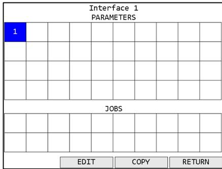
Press the button below **EDIT** to go to the Parameter Edit screen. The parameter number will remain white until the parameter has been successfully set up.
