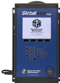
The Global 400mp is equipped with a color LCD display, four function keys immediately below the LCD, a numeric keypad with decimal point, navigation keys, and enter and escape buttons. The current function of the function keys is indicated at the bottom of the LCD above the button.
