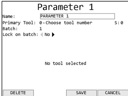
Press the down arrow to move the cursor to the Primary Tool row, followed by 1 to assign the tool to the parameter. Press ENT or the button below **SAVE** to save the changes and return to the Choose Parameter screen.
