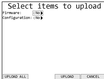
6. When the unit changes to the upload screen, it will search the root folder of the drive for the firmware update. If no valid update file is found, the screen will show an error. Otherwise, press the right arrow to select the firmware update and then **UPLOAD** to start the upload.
