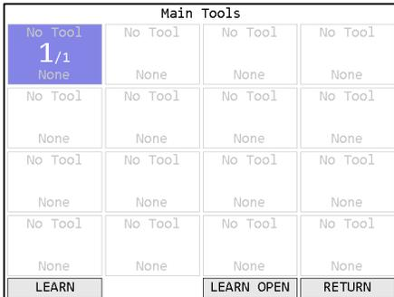
If the tool you are going to learn to the Global 400mp has previously been used with another unit, make sure the tool has been “forgotten” (radio disconnected) from that unit before continuing. Press the button beneath **LEARN** to begin the learn process.
